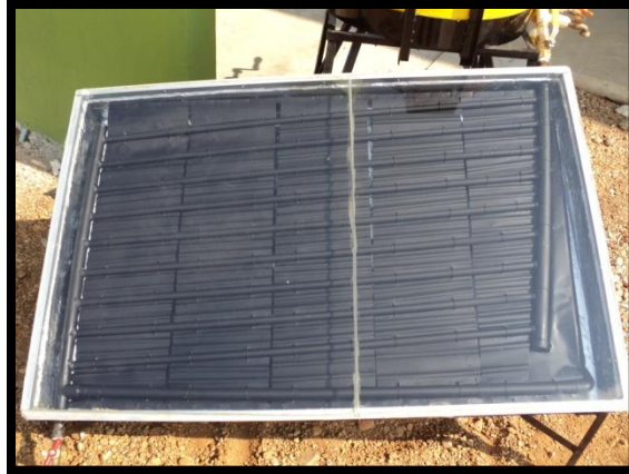
Figura 3.3. Colector solar del reactor
