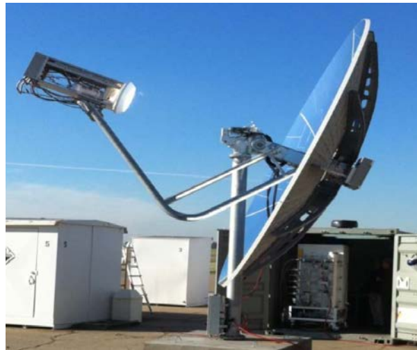
Figure 7. Sunexus solar reformer attached to a concentrating dish. Taken from [76].
