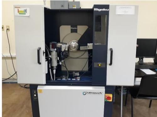
**Figura 10.** Difractor de Rayos X Rigaku Ultima IV.
